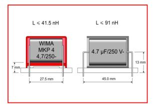
Figure 6: Comparison self-inductance axial vs. radial
