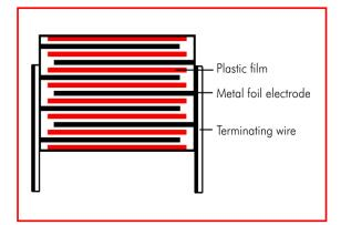
Figure 9: Cross section of WIMA FKP 3
