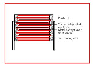
Figure 7: Cross section of WIMA MKP 4
