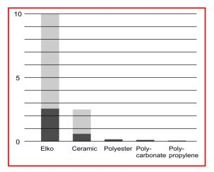
Figure 3: Dielectric absorption
