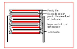
Figure 8: Cross section of WIMA MKP 10
