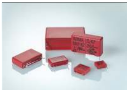
WIMA Capacitors Class X2, X1 and Y2 Dielectric: PP PCM: 7.5 mm to 37.5 mm Capacitance values: 1000 pF to 10 \mu\text{F} Voltage ranges: 300 VAC to 440 VAC
