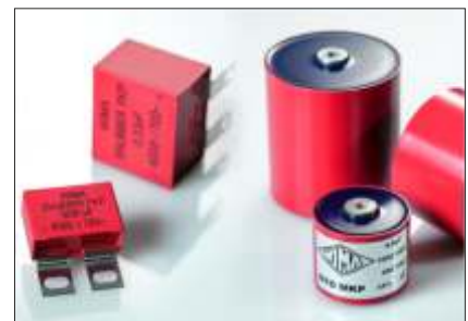
WIMA Snubber and GTO Capacitors Dielectric: PP Contacts: plates or axial screw connection Capacitance values: 0.01 \mu\text{F} to 100 \mu\text{F} Voltage ranges: 400 VDC to 4000 VDC
