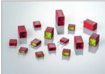
WIMA Capacitors with PCM 5 mm Dielectric: PET, PP PCM: 5 mm Capacitance values: 33 pF to 10 \mu\text{F} Voltage ranges: 50 VDC to 1000 VDC
