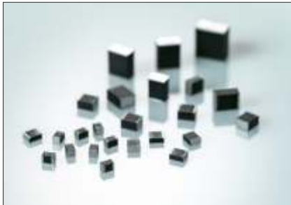
WIMA SMD Capacitors Dielectric: PET, PEN, PPS Size codes: 1812 to 6054 Capacitance values: 0.01 \mu\text{F} to 6.8 \mu\text{F} Voltage ranges: 63 VDC to 1000 VDC
