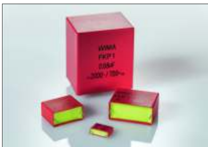
WIMA FKP 1 Pulse Capacitors Dielectric: PP PCM: 15 mm to 52.5 mm Capacitance values: 100 pF to 4.7 \mu\text{F} Voltage ranges: 400 VDC to 6000 VDC
