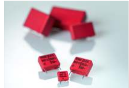
WIMA MKP 4 / MKP 10 Capacitors Dielectric: PP PCM: 7.5 mm to 52.5 mm Capacitance values: 1000 pF to 47 \mu\text{F} Voltage ranges: 100 VDC to 3000 VDC
